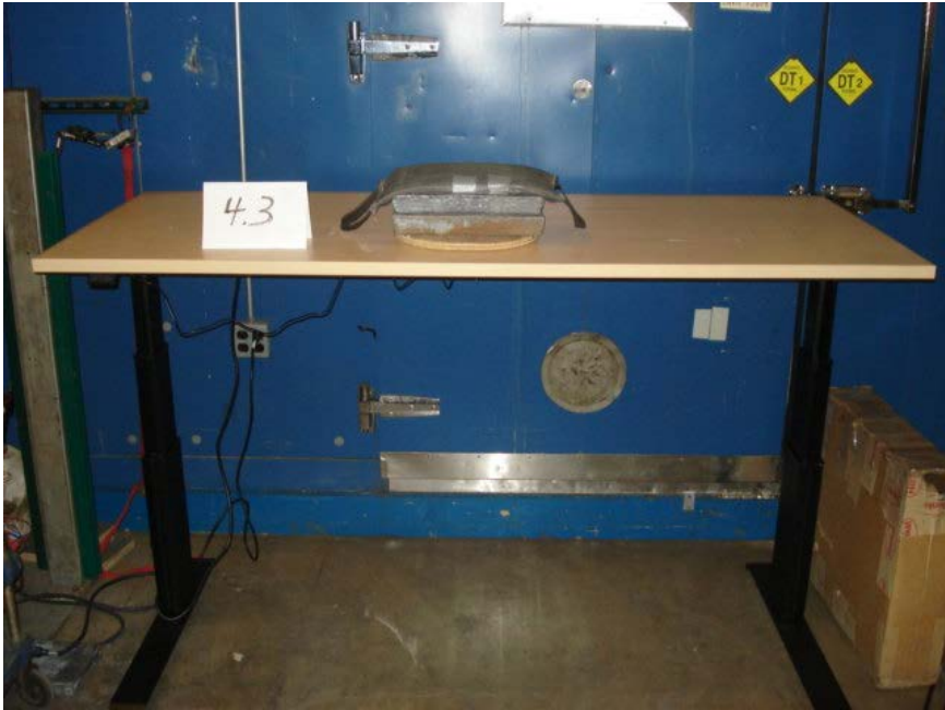
Photo No. 1 - Section 4.3 Stability Under Vertical Load Test
