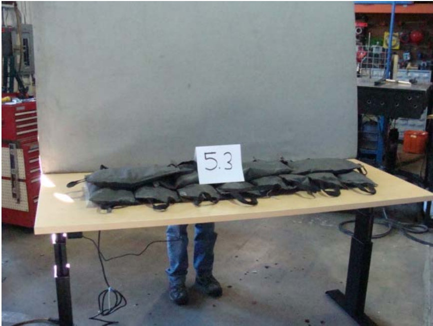
Photo No. 3 - Section 5.3 Distributed Function Load Test
