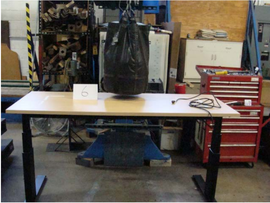
Photo No. 6 - Section 6 Top Load Ease Cycle Test
