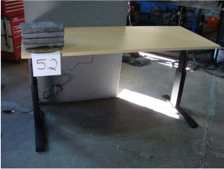
Photo No. 2 - Section 5.2 Concentrated Function Load Test
