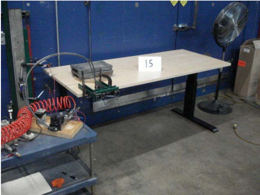
Photo No. 9 - Section 15 Work Surface Vertical Adjustment Test
