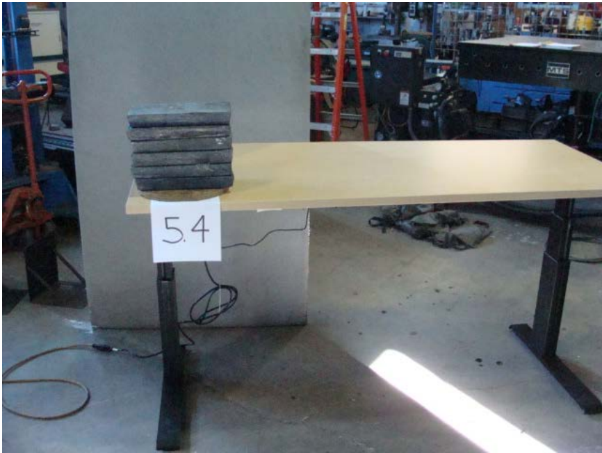
Photo No. 4 - Section 5.4 Concentrated Proof Load Test
