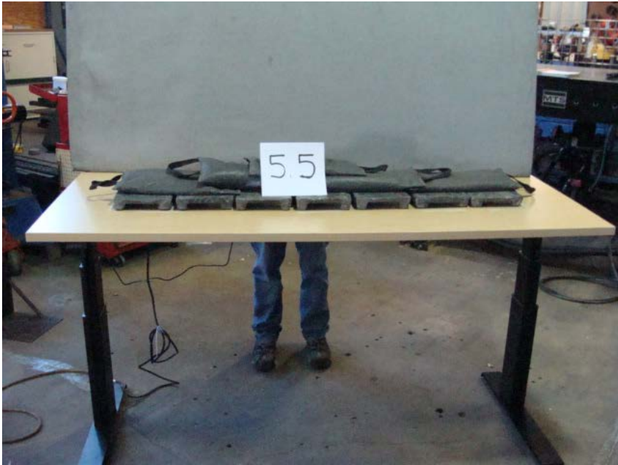
Photo No. 5 - Section 5.5 Distributed Proof Load Test
